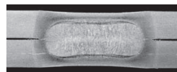
Sectional structure 1.6 mm, coating weight: 70/70 g/m 2
