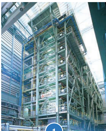
Annealing furnace (Vertical direct-fired reducing furnace)
