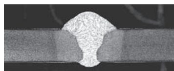
Sectional structure 3.2 mm, coating weight: 145/145 g/m 2
