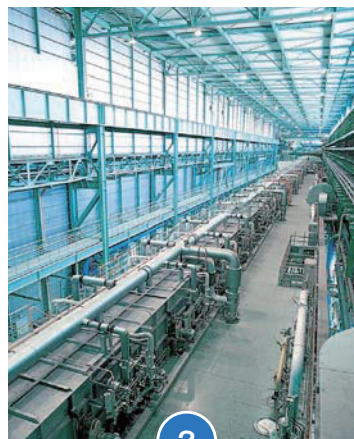
Annealing furnace (Horizontal radiant tube furnace)
